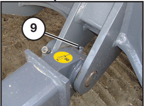
Dozer Pivot, left
