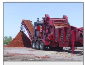
The B-66 can be equipped with the optional Rotochopper patented grind and color system for making perfect colored mulch in one pass.
