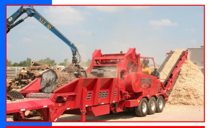
**Diesel or Electric Horizontal Grinder**
