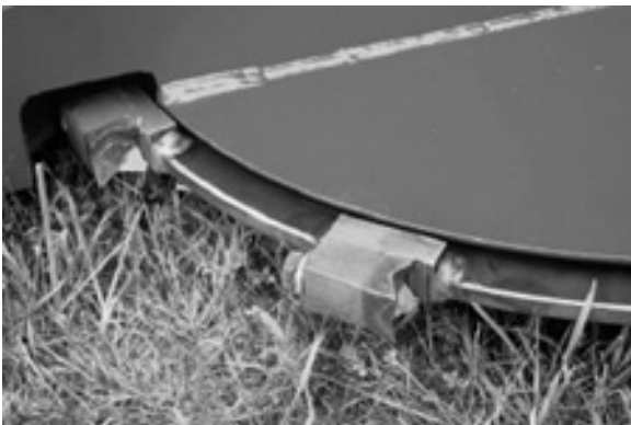
1" high tensile strength saw disc with 10 Quadco teeth
