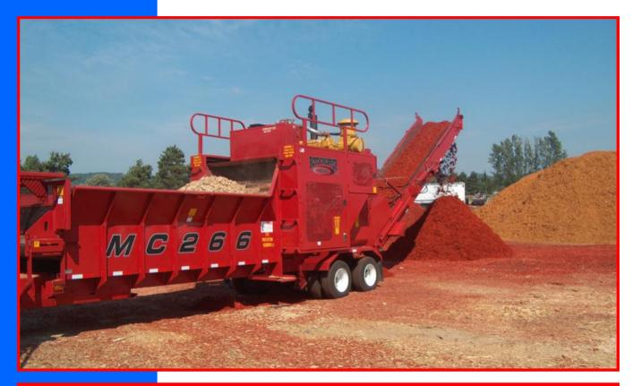
**Diesel-Powered Wood Grinding Systems**
