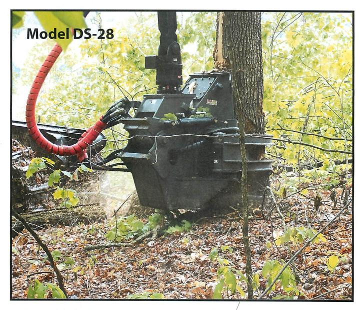
The DS-28 is a rugged chain and bar dangle saw. Designed for use on excavators, track feller bunchers, and loader type carriers. The durable and cost effective DS-28 runs on auxiliary or standard bucket hydraulics. It is great for general logging, pulp production, thinning, right of way clearing, storm clean up and more!
