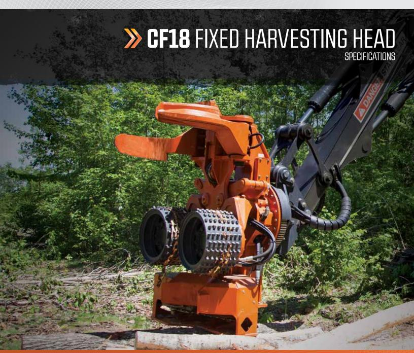
The Barko® CF18 fixed harvesting head provides optimal performance on a wide range of harvesting and processing applications. Featuring a patent-pending design equipped with IQAN® control system, onboard valving and center hose routing, the CF18 is precisely engineered for fast and efficient cutting and delimbing.
